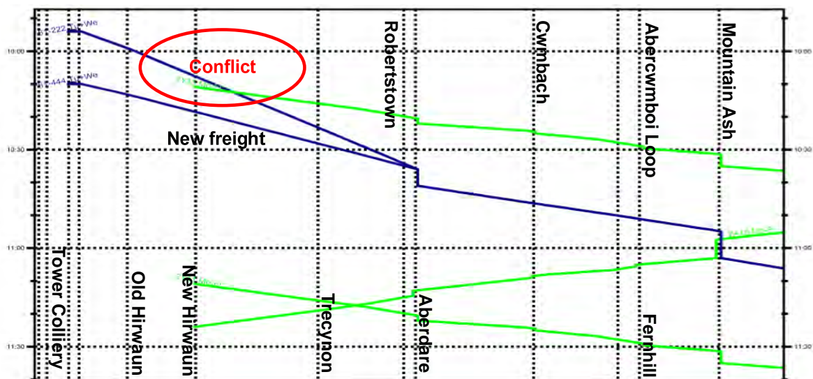
Figure 3: Train Graph extract from RailSys showing where the passenger and freight trains would conflict. (The x-axis shows the locations and the y-axis shows time.)
